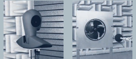
Room for precision noise measuring
